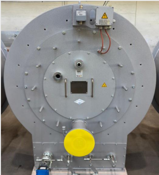
Fig. 9: Ray Gas Burner
