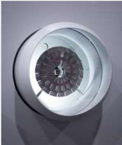
Fig. 4: RAY Oil pressure atomizer PDE-K, KVA Delfzijl, Netherlands
